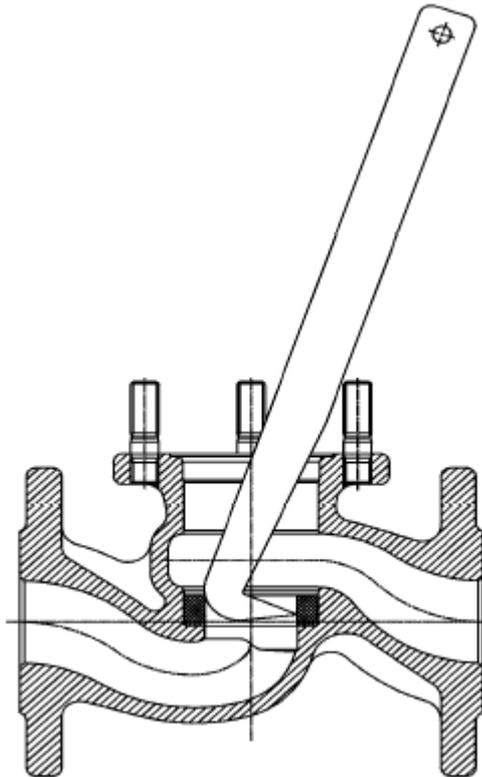
Removing of the graphite sealing ring with special tool, for the removing of the Lantern bush, please use a proper puller.
